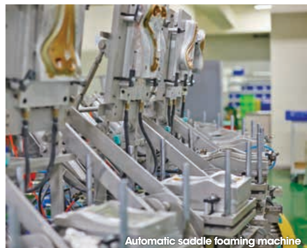
Automatic saddle foaming carousel machine
